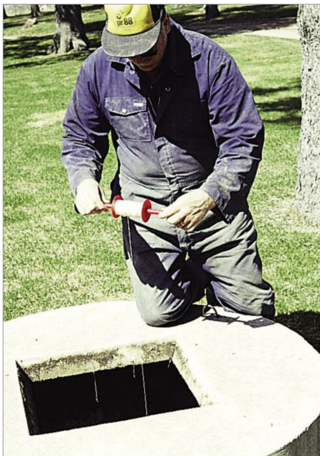
Figure 4. Measuring the depth of water in a private water well.
