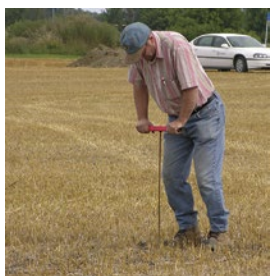
Photo 8–3a. Identify parts of the field with potential compaction problems by using a tile probe or flexible rod.
