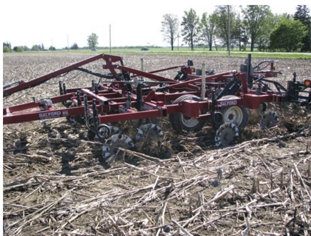
Photo 1–1. Vertical tillage tools are designed to manage and mix residue with light soil fractioning.
