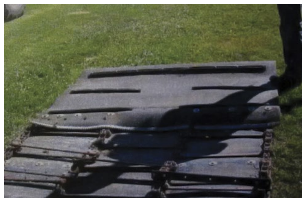
Photo 7–1. Use rubber belts to prevent plant fibre from wrapping around shafts, chains, etc. Courtesy of Manitoba government.
