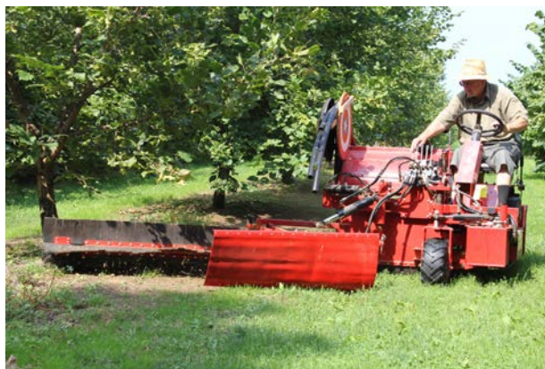
Figure 8-3. A compact harvester picking up ripe hazelnuts under trees. The rotating sweep paddles extend underneath the large canopy.
