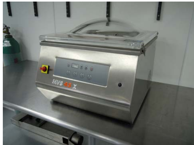
Figure 8-5. A commercial vacuum packaging unit is used to maintain kernel quality and prevent oxidation of nut oils during cold storage.
