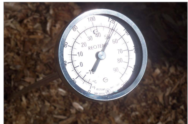
Figure 3. Long-stem thermometer inserted in compost pile recording a temperature of 51°C (124°F).
