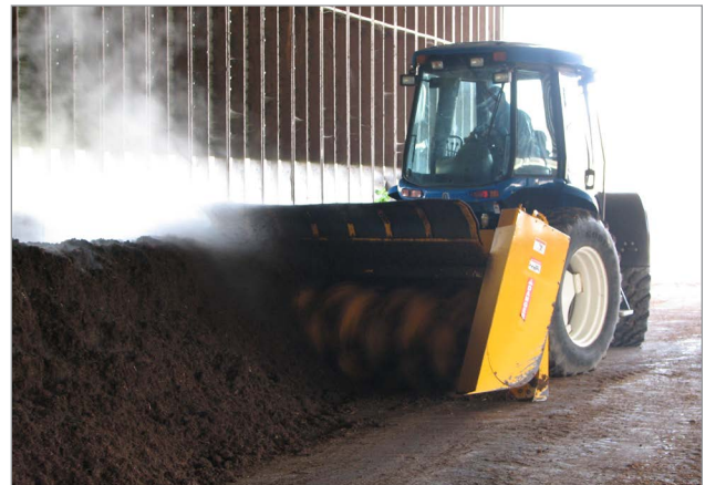
Figure 1. Brown Bear windrow compost turning unit and a windrow of poultry carcasses and substrate materials.
