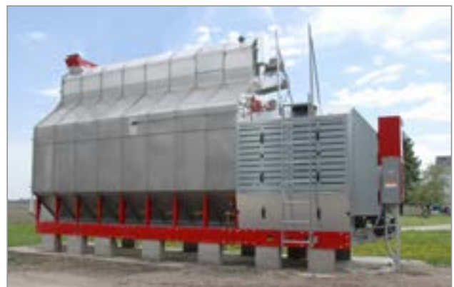
Figure 1. A typical grain dryer. This is a horizontal continuous cross-flow grain dryer without heat recirculation. Source: Brock Grain Systems, Milford, Indiana, USA .
