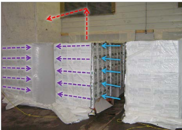
Figure 2. Tunnel horizontal airflow system example.
