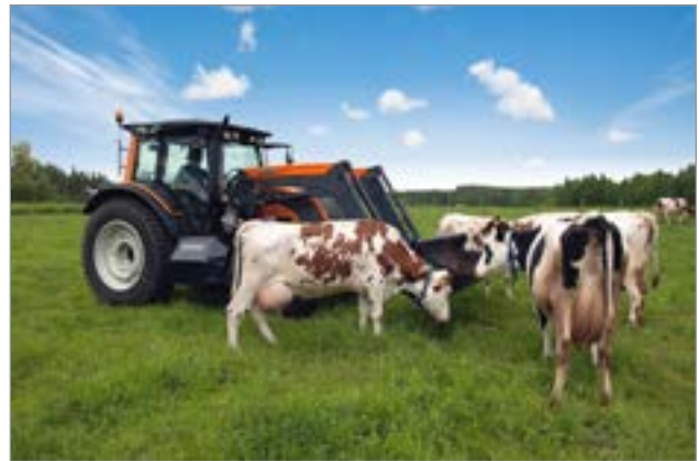
Figure 3. A prototype biogas tractor that runs on farm-based biogas. Note the pressurized biogas storage system on the lower side of the tractor. Source: Valtra and AGCO.
