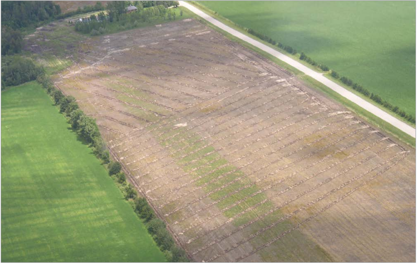
Figure 1. Aerial view of a recently installed subsurface drainage system.
