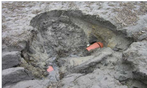
Figure 6. Drain pipe blowout.
