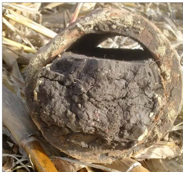
Figure 8. Old clay tile filled with sediment.
