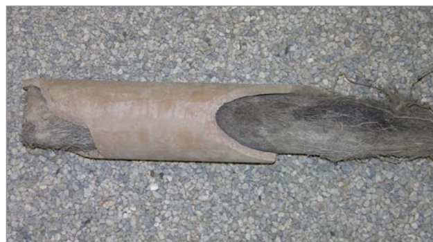
Figure 5. Drain pipe plugged with tree roots.
