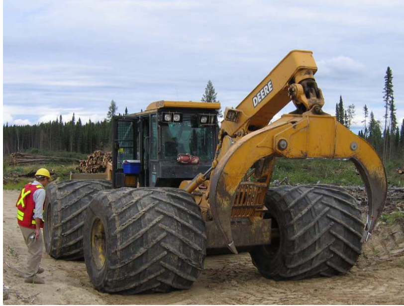
Figure 5.2j. Using machinery with low ground pressure options, such as these high floatation tires, can help to minimize damage and may expand the range of sites on which operations can occur in unfrozen conditions (photo by Joe Maure).
