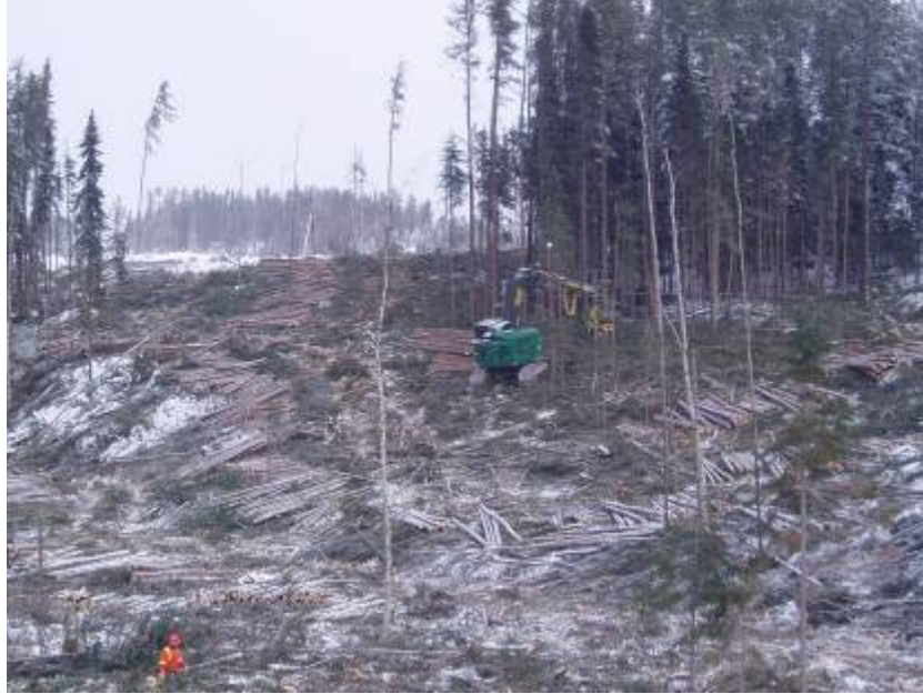
Figure 5.2h. A cut-to-length harvester can be used to de-limb and slash trees at the stump to avoid moving nutrients associated with unutilized fibre to roadside (photo by Mike Curran).
