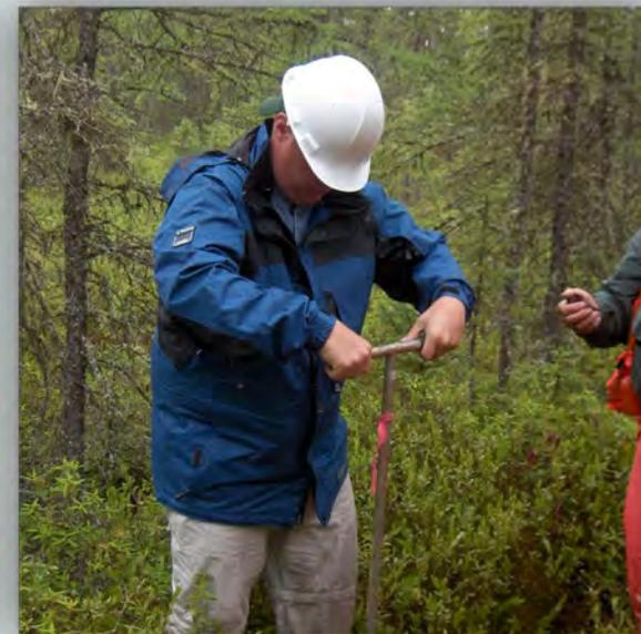
using soil auger
