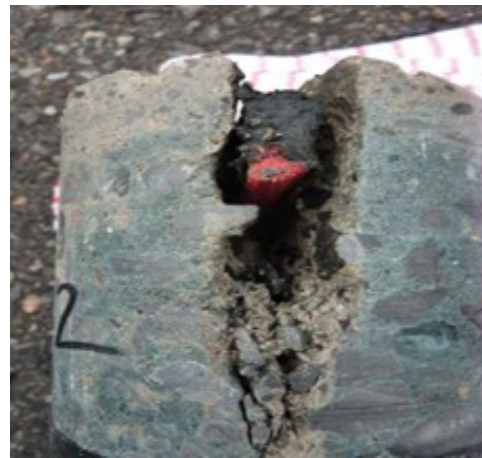
Figure 7b: Concrete joint deterioration shown in core sample.
