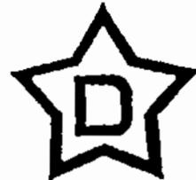
This symbol indicates the extinguisher is applicable for use on certain combustible materials such as sodium, magnesium, potassium, etc. The background of the symbol will be either metallic or yellow.
