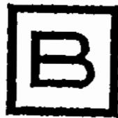
This symbol indicates the extinguisher is for use on flammable gases, greases or similar materials. The background of the symbol will be either metallic or red.
