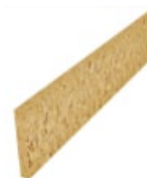
Figure 5. Laminated strand lumber [4]
