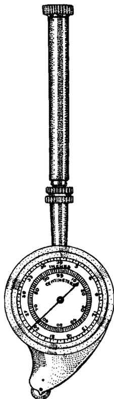
This unit measures linear distance in centimetres or inches. The indicator needle is set at zero by rotating the tracing wheel. Measure the shoreline by tracing the outline of the figure, and then read the result from the scale. Care must be taken so that the indicator needle travels in a positive direction. Also, on a large lake the needle may travel more than once around the circumference of the dial. Therefore, the operator should keep close watch as to the number of revolutions.
