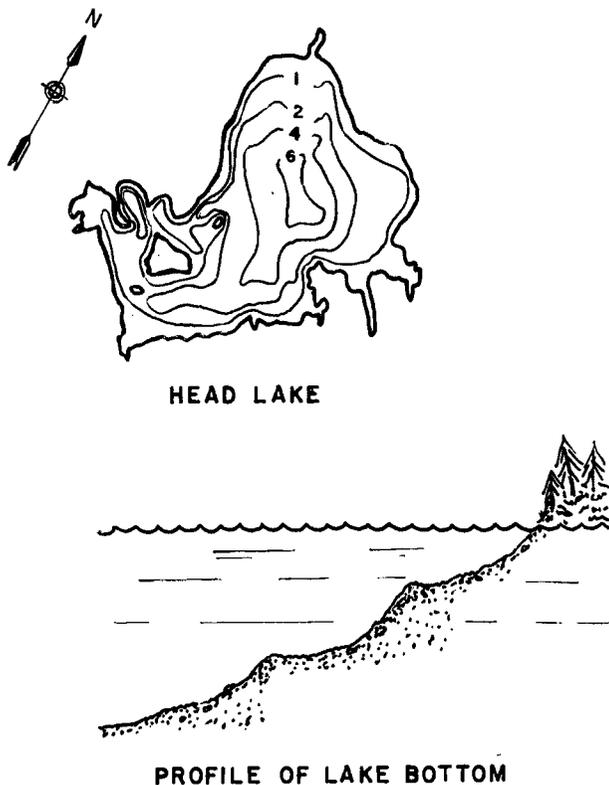
The Contour Map, sometimes called a Bathymetric or Hydrographic chart is a graphic representation of the lake bottom or lake bed, as determined from depth soundings. The Contour Map reveals the extent of shallows, the degree of inclination of the lake bottom, the shoals and the deep holes. To prepare the Contour Map, the various depths of the water basin have to be measured by an echo sounder.
