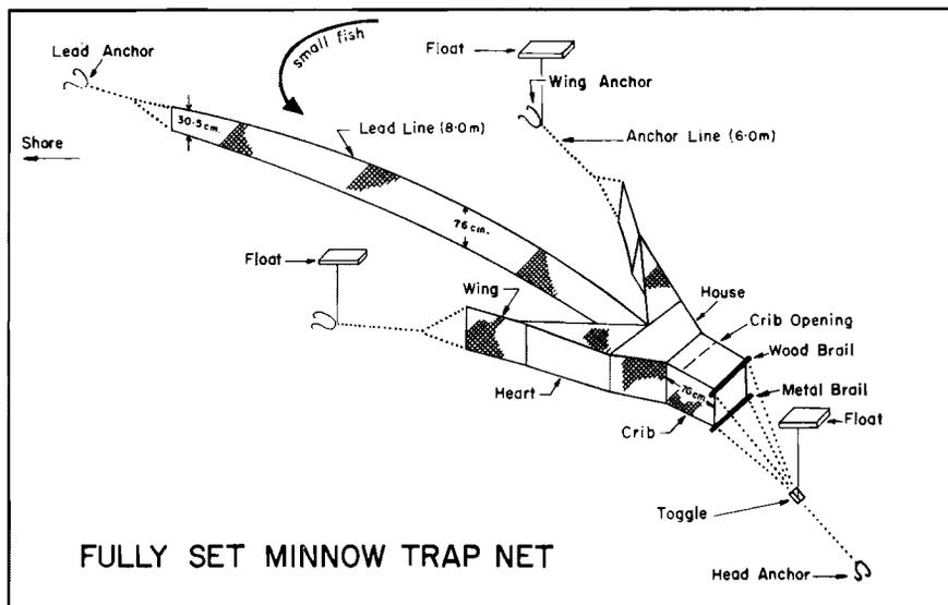
The net is usually set perpendicular to shore with the crib section completely submerged in the deeper water, but not in a water depth exceeding double the net height of five feet (1.5 m).
