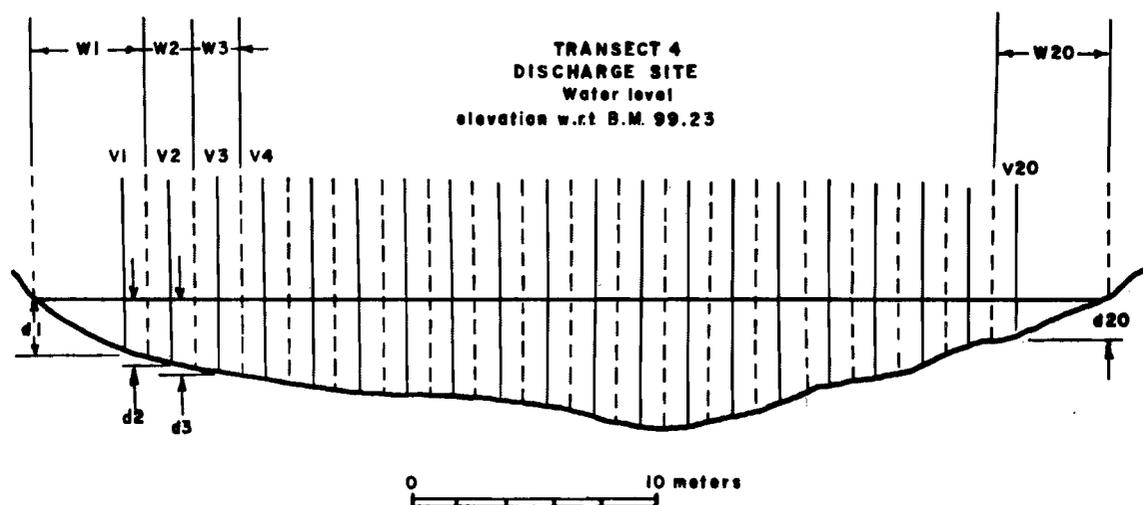
The total depth and the water velocity are measured at each vertical. If the water depth is 1 m or less, then the velocity is measured at the proportion 0.6 of the total depth. If the water depth is greater than one metre then two velocity measurement are taken at the proportions 0.2 and 0.8 of the total depth. The average velocity is calculated as:
