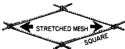
The stretched measure of the mesh sizes will vary at regular  $12.5 \pm$  millimetres (0.5 inch) intervals between 25 mm (1.0 in.) and 140 mm (5.5 in.).
