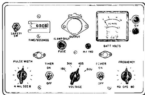
Due to the decreased mortality rate and faster recovery rate of the shocked fish, *pulsed direct current* operation of the unit is recommended. In view of the catchability efficiency of other types of gear in lakes and the high unit price tags, the electrofishing method is presently confined for use in the stream survey.
