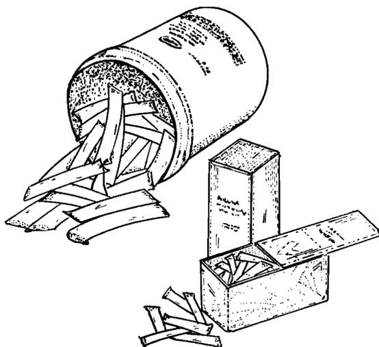
Whether the Hach DR-EL or AL36 kit is used, the dissolved oxygen test procedure is identical. Pre-measured dry powdered Manganous Sulphate (D.O.I), Alkaline Iodide-Azide (D.O.II) and Sul-famic Acid (D.O.III) pillows are used. Each pillow contains sufficient reagent for one test. The polyethylene container is easily opened with clippers or a sharp knife. The dissolved oxygen content is determined by adding Phenyl Arsine Oxide (P.A.O.) solution.
