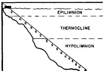
The other method is a hanging set, with only one terminal anchored. It is preferable to set it in such a way that the float terminal is near and secured to the shore and the line suspended near the basin rim from bottom to surface.
