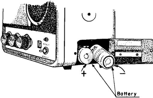
The power supply for both the Furuno and Ferrograph units is a 12V battery (wet or dry cell). Each unit normally has a volt-meter dial to indicate the power supply strength. Furuno models should operate as efficiently with eight *transistor* dry cell batteries as with twelve volt wet cells. You can expect problems though if you use ordinary flashlight batteries.
