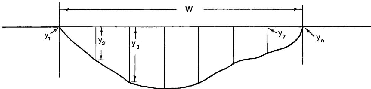
$$\begin{aligned} \text{Mean Depth (Transect \#1)} &= \frac{\frac{Y_1 + Y_2}{2} + \frac{Y_2 + Y_3}{2} + \dots + \frac{Y_{n-1} + Y_n}{2}}{\eta - 1} \\ &= \frac{\frac{0.05}{2} + \frac{0.16}{2} + \dots + \frac{0.04}{2}}{7} = 0.07 \text{ m} \end{aligned}$$
