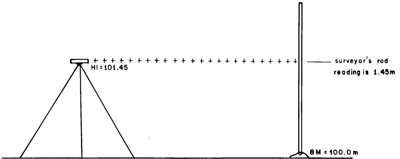
**Height of the Instrument (HI):** The HI is always the result of a backsight and is the sum of the known elevation and the BS rod reading.
