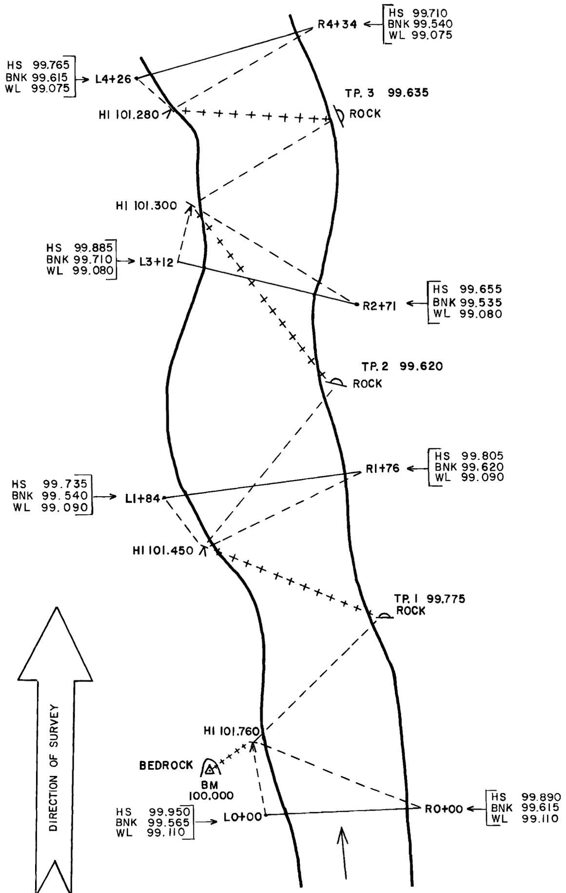
**PATH AND DIRECTION OF SURVEY SHOTS AT A TYPICAL STATION**
