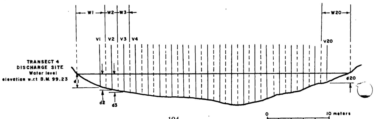
In the preceding diagram of a discharge measuring site, note that the solid vertical lines denote the measuring points for velocity ( $v$ ) and depth ( $d$ ). The broken vertical lines denote the limits of the panel width ( $w$ ). The panels W1 and W20 are both wider than the others to compensate for the edge effect of laminar flow.
