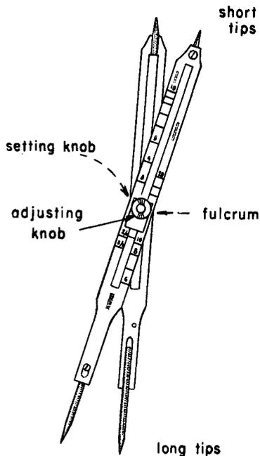
Proportional dividers are instruments made of crossed double pointed metal arms. They are made in such a way (as the name suggests) that they can be adjusted to measure ratios or proportions.
