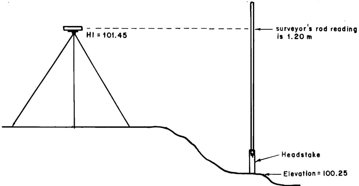
**Turning Point (TP):** The turning point is a temporary bench mark upon which FS and BS readings are taken to continue a line of levels. This is necessary where a shot may be too long or where there is an obstruction between the instrument and the point to be measured.
