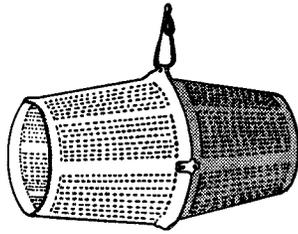
a) The Anglers Minnow Trap Net: A two sectioned unit of wire or plastic mesh with small throat openings at either end and which lock together to form a trap.
