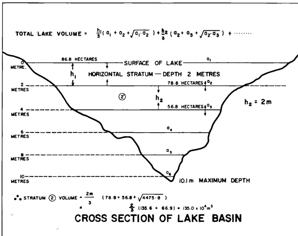
To calculate the volume of a lake, measure the surface area of each contour. Then, by applying the formula above, the volume is calculated. These calculations are done by computer at Main Office or can be done at field offices using a programmable calculator.
