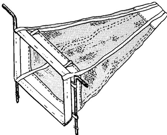
The drift net consists of a rectangular metal or wooden frame on which a nylon net is attached. Two stakes attached to the frame hold the net into the substrate. The net passively collects invertebrates that are carried along in the current (drifting).
