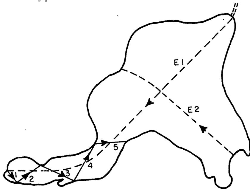
"E" Lines dictate sounding density: — The more irregular the bottom profile, the greater the number of transect lines required. It is mandatory that the lake be adequately covered by sounding lines but doing too many only wastes time and energy.
