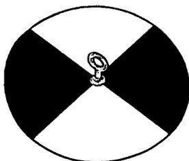
Transparency in lakes is measured with a weighted metal disc, twenty centimetres in diameter with alternate white and black quadrants. This instrument is known as a *secchi disc*. A line, graduated in metres and centimetres is attached to the disc.
