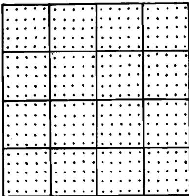
There is more than one dot grid design, but all are of the same principle. A one hundred dot per square inch transparent overlay can be used on any scale map.
