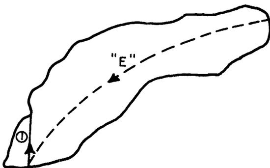
The "E" Line is an exploratory line and will always be the initial line run. If the basin shape is simple (reasonably oval or rectangular without indentations (bays)), then one "E" Line will normally suffice. If the basin shape is more complex, then more than one "E" Line is required. "E" Lines will be run the length of the basin or basin segment, midway between the shorelines. It may not, and it does not need to be a straight line. It will be shown as illustrated on the transect map.
