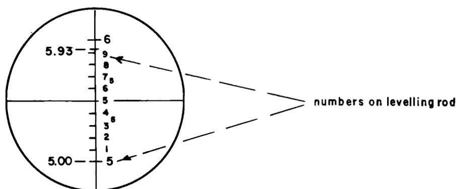
The distance from the level to the rod is determined by reading the rod heights that the stadia cross-hairs have intersected. Subtract the lower reading from the upper reading and multiply by a constant (usually 100, but this may vary with different instruments). For example, upper and lower stadia readings of 5.93 and 5.00 m, respectively, indicate that the rod is positioned 9.30 m ( $0.93 \times 100$ ) from the level.
