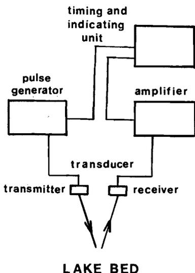
There are a number of models and types of echo sounders, but all operate on the same principle — 'sonar'. This word is derived from *sound*, *navigation* and *ranging*. Simply, sonar measures and records time between the transmission of sound through water and the reception of an echo. A schematic diagram of the principle is shown.
