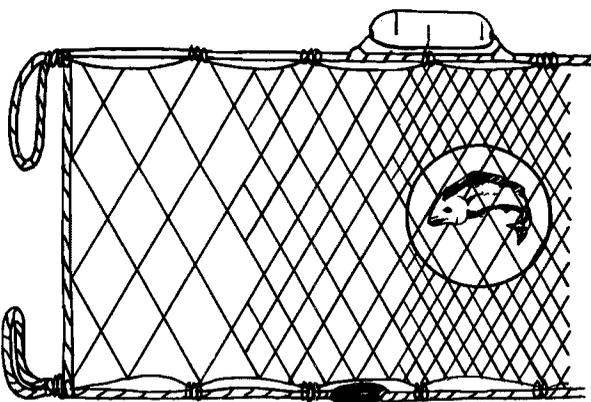
Experimental gangs of either multifilament (nylon) or monofilament nets, are used for sampling larger fish. The recommended minimal *gang of nets* consists of at least eight different stretched mesh size segments of 1.5 metres in depth and fifteen metres in length. The continuing use of the eight by fifty foot nets in one-half inch intervals is logical and practical, until replacement is required, or until the equivalent metric sized nets are available through suppliers.
