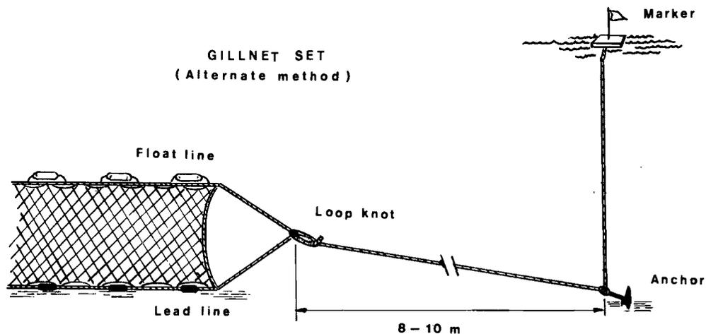
The net should not be set on steep slopes nor across drop-offs. Sites of this nature result in narrowing or closing of meshes which prevent gilling.
