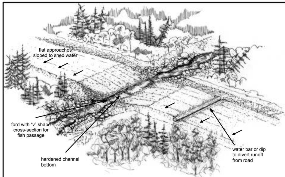
**Figure 5.1e. Typical features of a ford (Illustration by Kestevan Design).**
