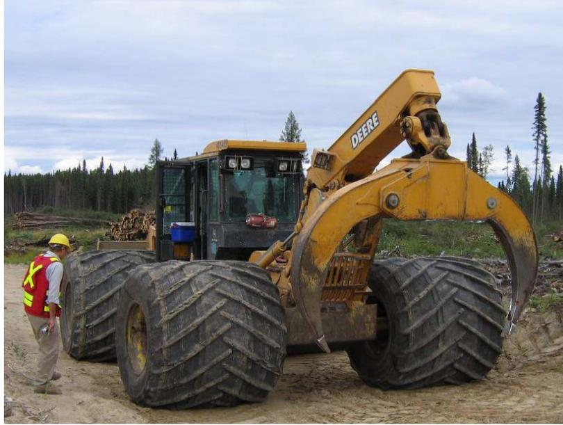
Figure 5.2j. Using machinery with low ground pressure options, such as these high flotation tires, can help to minimize damage and may expand the range of sites on which operations can occur in unfrozen conditions (photo by Joe Maure).
