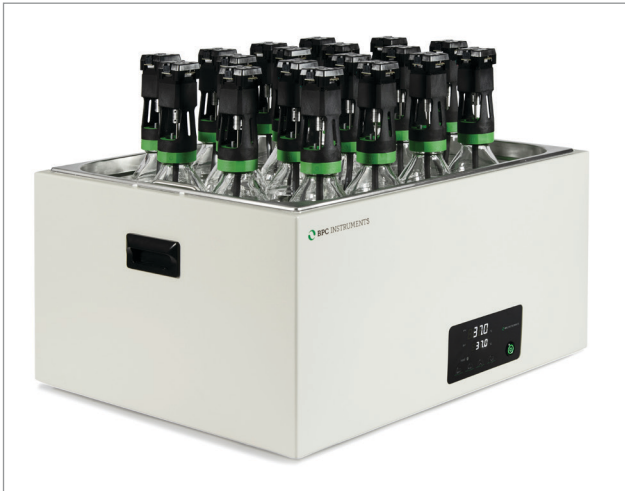
Figure 2. A thermo bath with 1-litre bottles is used to determine potential biogas yields of various substrates. Source: BPC Instruments .
