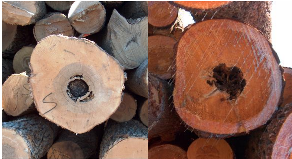
Figure 5 - Examples of heart rot
