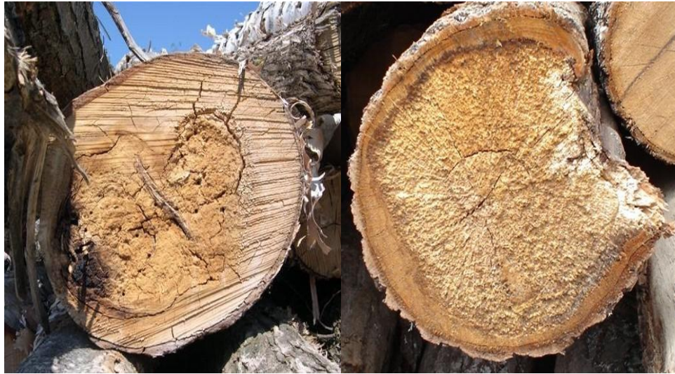
Figure 9 - Examples of punk rot
