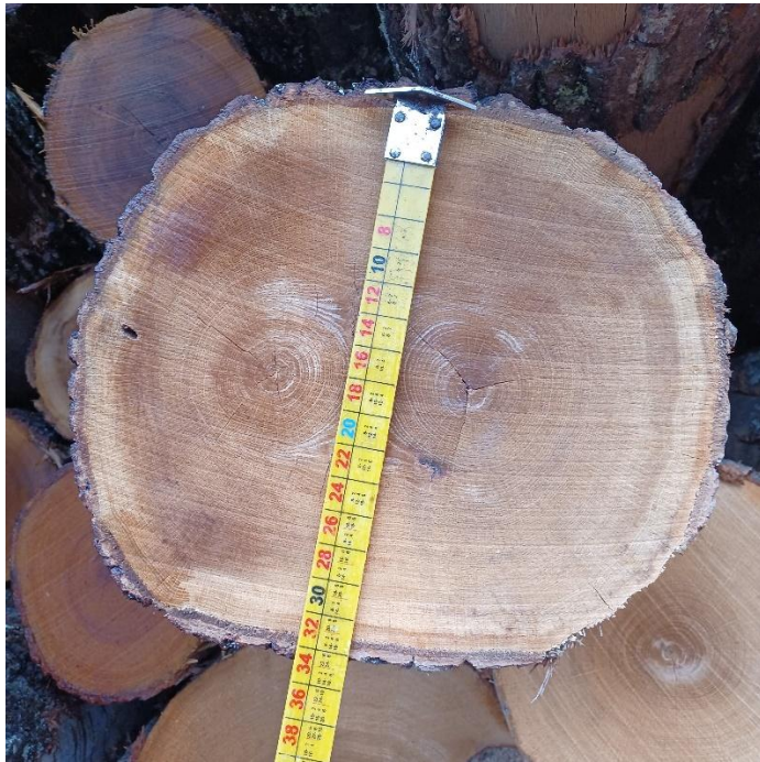
Figure 3 - Measuring diameters when cat's eyes are encountered
