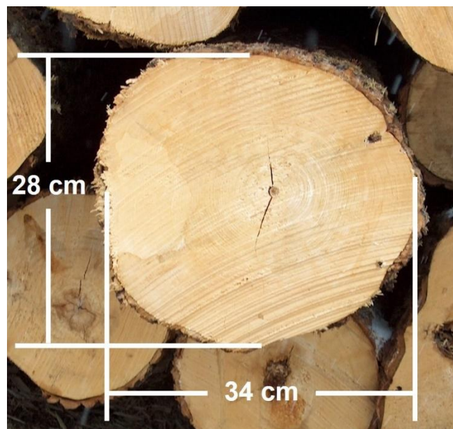
Figure 2 - Measuring diameters: logs with irregular sawn surfaces
