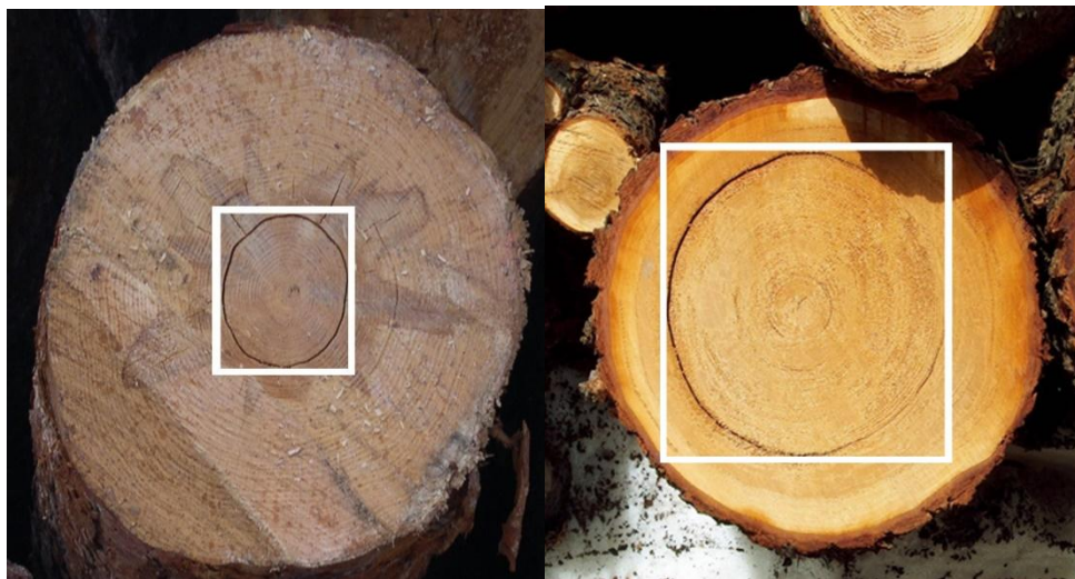
Figure 8 - Examples of shake
